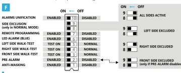
ATTENTION: THE SENSOR IS OPERATIVE ONLY WITH THE INSERTED COVER! After each modification of dips and trimmers it is necessary to close the cover and wait at least 3 seconds during which the sensor reads the settings.
