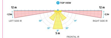
Left and right detecting sides are 12 meters length range each, reaching 24 meters of linear protection, with 10° opening angle on horizontal plane.
