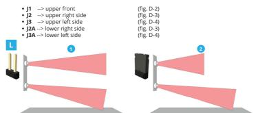
When the jumper is inserted, the range and sensitivity of the head is reduced by about 50% respect to the maximum value (the maximum value depends on the trimmer adjustment). The trimmers always adjust the range of both heads (upper and lower) of the corresponding
