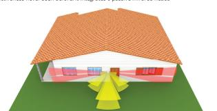
A double IR barrier on the sides of the sensor creates a protection for doors and windows placed on the front of a building for a length of 12 + 12 meters. The lateral detection on each side is entrusted to the combination of two IR heads with AND logic, which generate two curtain detection zones with 10 ° opening and range up to 12 meters each.
