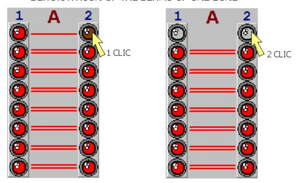
This figure is a simple representation of the bidirectional beams in which the round spheres are the infrared TXs.
