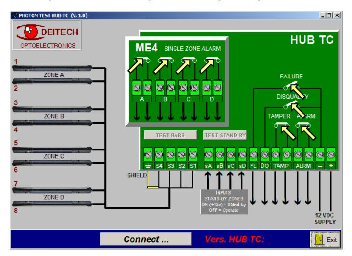
To execute the test of the STANDBY inputs (active +12V)
