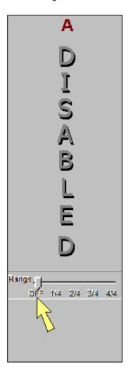
The Zones (pairs) <u>not</u> used may be disabled by moving the sliding cursor to the OFF position. To confirm the disabling of the relative Zone, the display will show the "Disabled" message.
