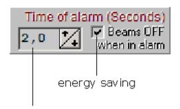
This regulation manages the temporization of the normally closed alarm relay. The opening of the contact in alarm stage can be adjusted from a minimum of 0,2 seconds up to a maximum of 10 seconds with steps of 0,2 seconds
